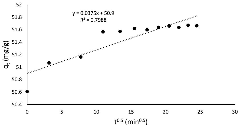
585 **Fig. 10** Intra-particle diffusion adsorption kinetic of Co onto the soil
