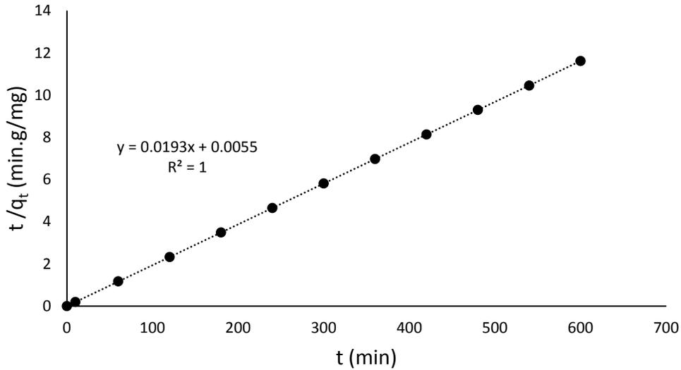
562 **Fig. 8** Pseudo-second-order adsorption kinetic of Co onto the soil
