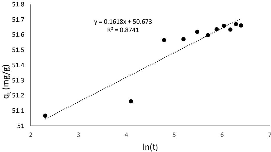
569 **Fig. 9** Elovich adsorption kinetic of Co onto the soil
