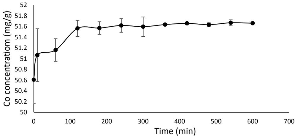
**Fig. 2** Effect of contact time on Co adsorption by soil
